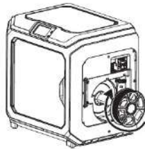
3. Notice: For filament convenient rotation, please install filament follow the direction shown in the picture.
