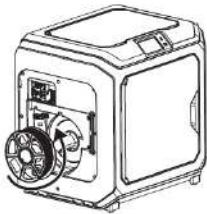
3. Notice: For filament convenient rotation, please install filament follow the direction shown in the picture.
