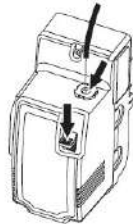
5. Press the spring presser, put filament vertically into the left filament intake to the bottom.
